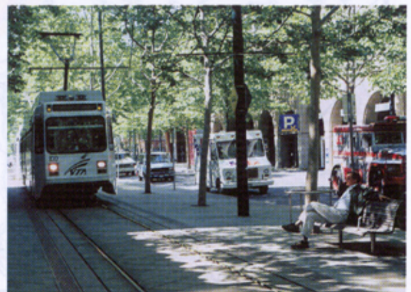
The photo above illustrates the use of an at-grade light rail transit line to serve a community's commercial district.
