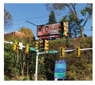
As part of this project, many intersections received new signal controllers or controller assemblies and emergency vehicle preemption. SR 68/356 & Hansen Ave intersection received a full signal upgrade. Global Positioning Satellite antenna and receivers were installed at multiple intersections to allow for time-based coordination. Coordination of traffic signals is one of the most cost effective ways of improving traffic flow along a corridor.
