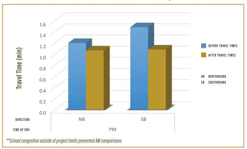
Prior to this SINC-UP Project, motorists typically experienced frustration of consecutive stopping at traffic signals due to the uncoordinated signals. This retiming project coordinated the traffic patterns through these intersections which alleviated consecutive stopping and reduced the motorist's frustration. This project also implemented a school timing pattern to accommodate the school zone between intersections.
