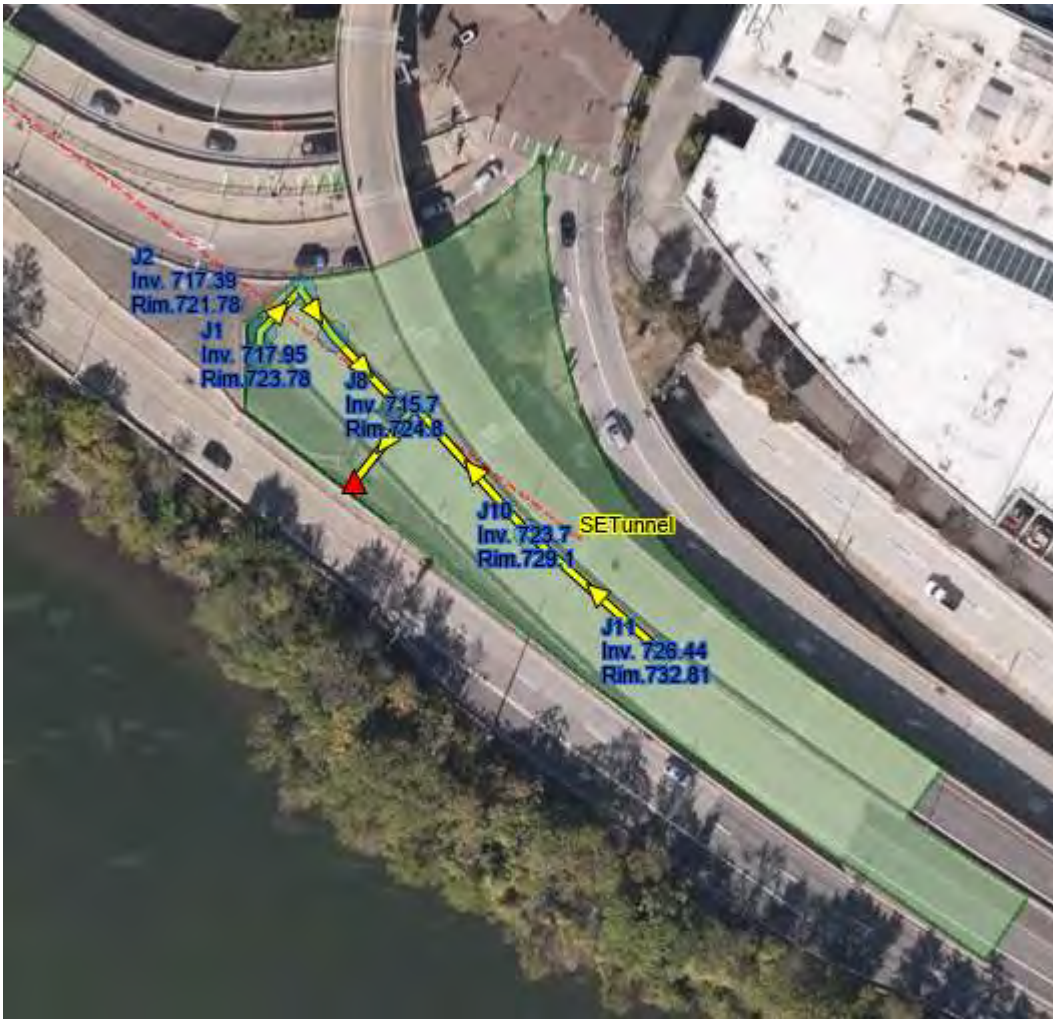
Figure B-20. Drainage area Southeast of Ramp D Tunnel Accounted for Flow to the Big Bathtub.
