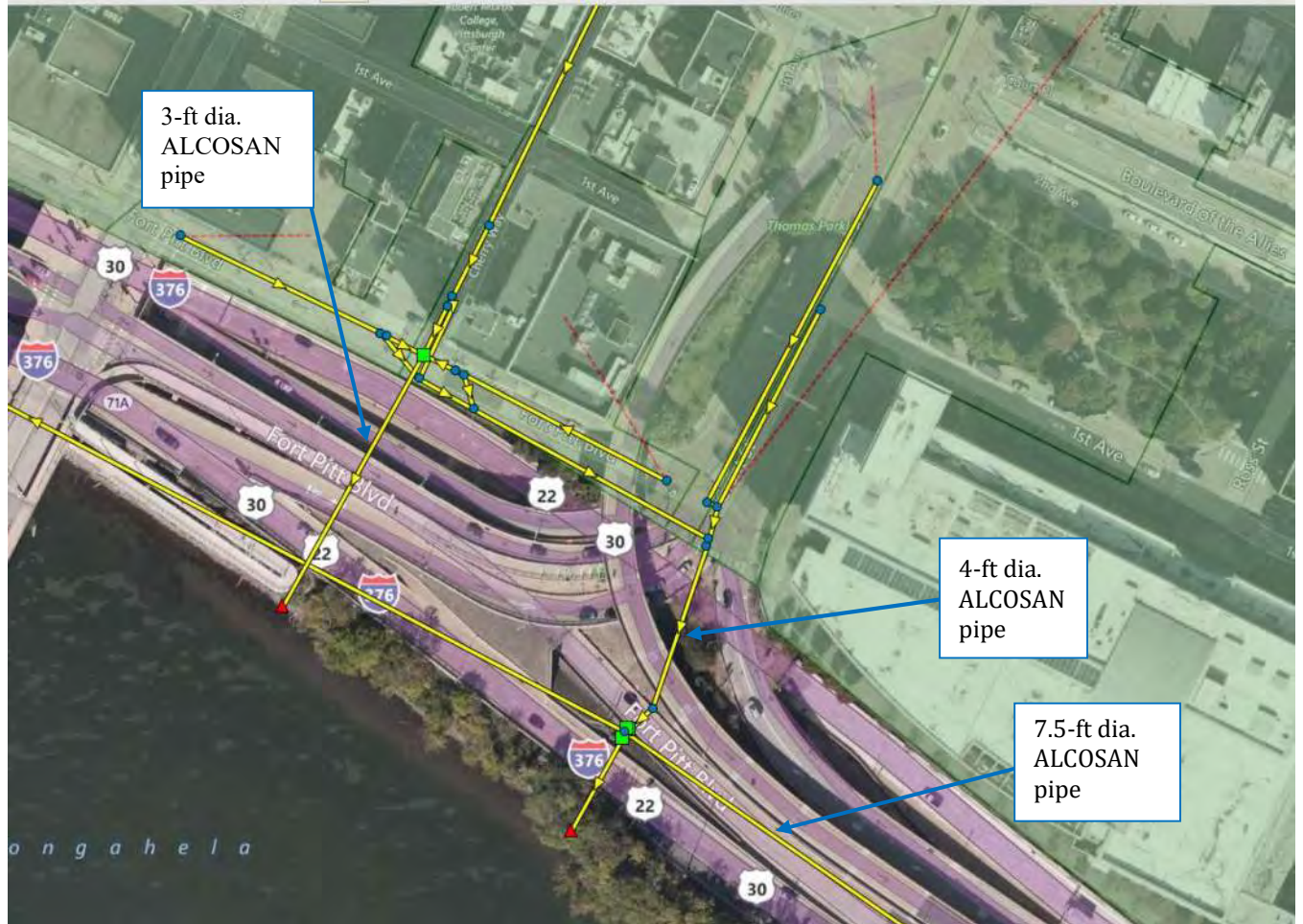
Figure B-5. ALCOSAN System Layout Through the Ramp D Area as Portrayed by the ALCOSAN SWMM Model
