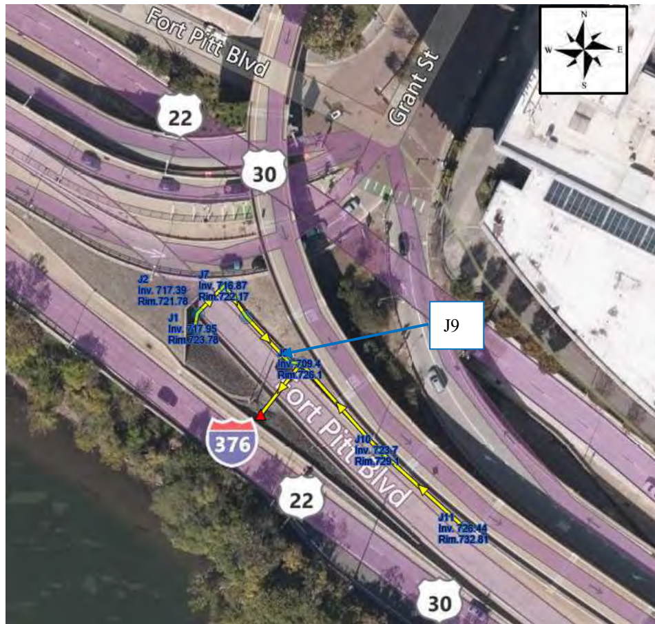
Figure B-21. PCSWMM Model of the Area Southeast of the Tunnel
